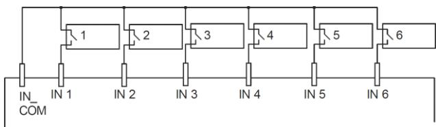
The IN1 to IN6 input cable length should not exceed **50 m (164 ft)**.
