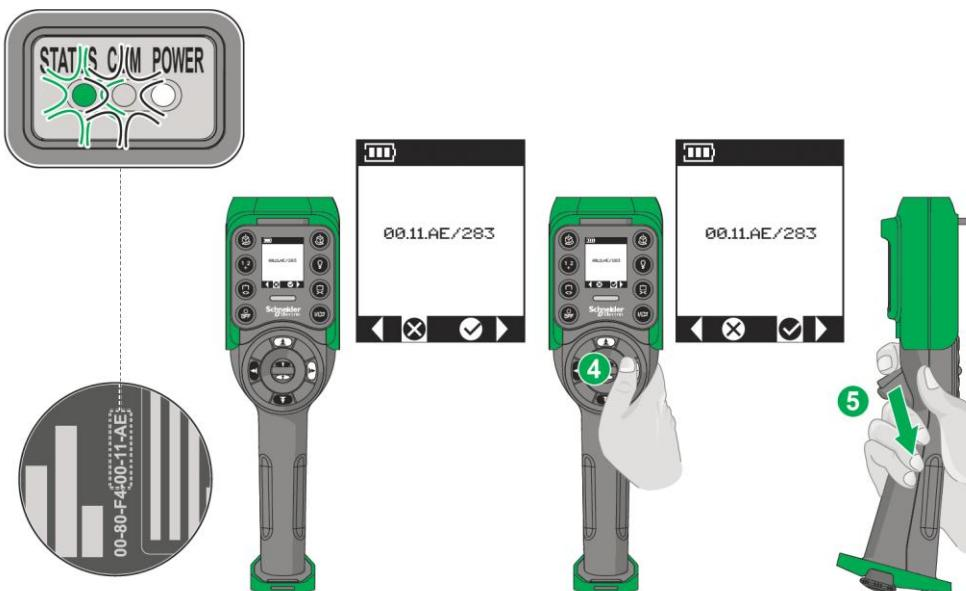
During pairing procedure of a Base Station with a Remote Device, the Base Station is signaling a feedback by the blinking of 'Status & Com' LEDs, to be sure that the correct Base Station is being paired. The operator must confirm or cancel the pairing procedure thanks to the Remote Device according to the Base Station feedback.
